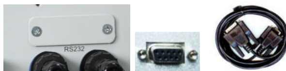
Fig. 10 RS232 serial port and special RS232 cable
