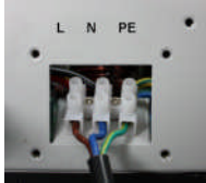
Fig. 8 AC terminals under AC terminals cover
